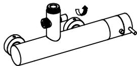
Turn the handle manually counterclockwise (as shown above), until the whole handle falls off.
