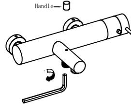
Use the 8mm allen key counterclockwise and rotate the G1 / 2 outlet joint part (as shown above, until the entire G1 / 2 outlet joint falls off
