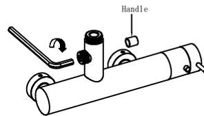
Use the 8mm allen key counterclockwise and rotate the G1 / 2 outlet joint part (as shown above, until the entire G1 / 2 outlet joint falls off
